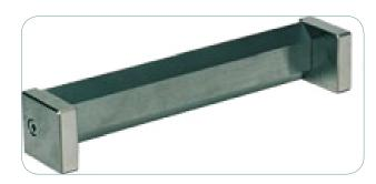
Applicator for the preparation of uniform films of coating materials, adhesives and similar products on plane substrates for testing purposes.
