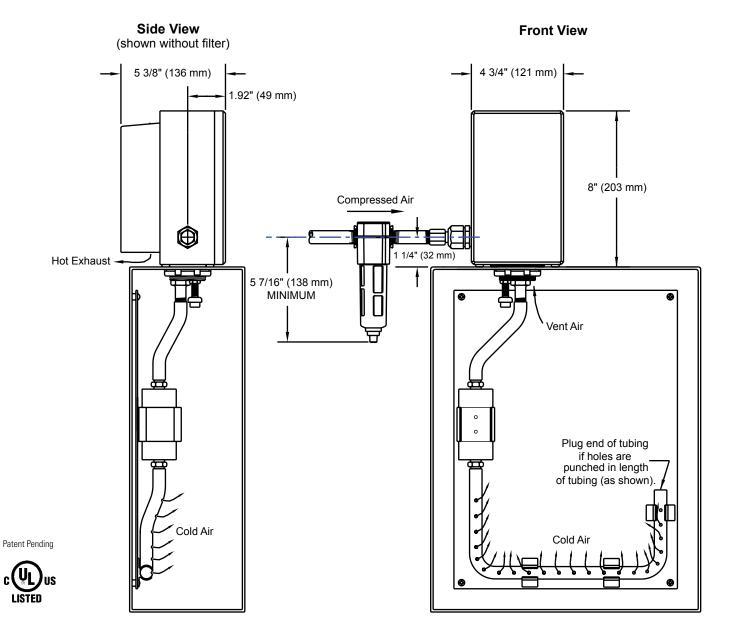
Vortec offers a complete line of Vortex Coolers for NEMA 12, 4 and 4X electrical cabinets. For assistance in sizing an appropriate Vortex A/C for your enclosure or for more information on any of our cooling models, please call our technical service staff at the number below.
