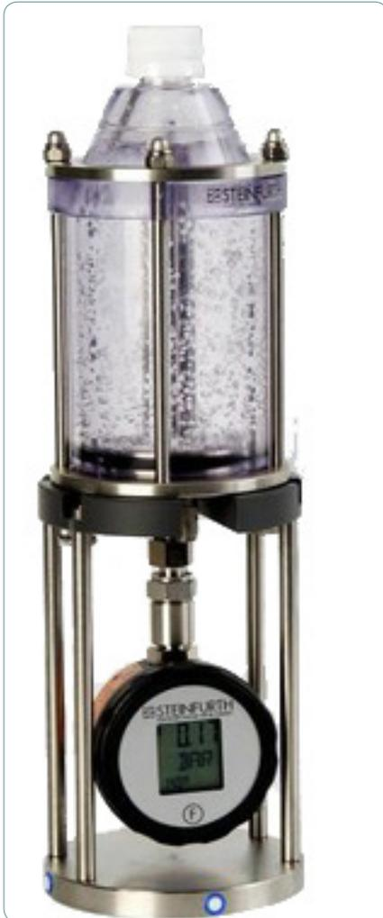
The Check Bottle TS 94.5 is used for monitoring the accuracy of the measuring heads of the CO<sub>2</sub> tester TS 91.7. It consists chiefly of a polycarbonate container and an integrated digital precision instrument, combining manometer and thermometer.
