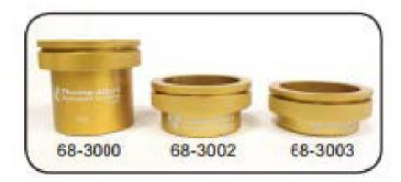
The Vapometer is used for determining the water vapor permeability of sheet materials such as specialty paper grades, polyethylene, building material, leather, weatherproof clothing, vinyl, foil, laminates and other thin sheet materials. This property is essential in determining if a material is moisture proof or has the ability to protect contents from the transmission of water vapor.
