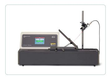
The most versatile peel tester on the market, the ChemInstruments Adhesion/Release testing machine with digital display is designed to perform PSTC, ASTM, TLMI, FINAT, and AFERA adhesion and release testing procedures.
