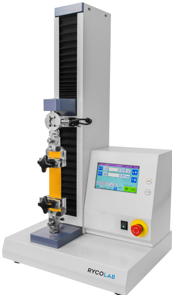
Figure: Tensile tester with manual clamps and touch screen
