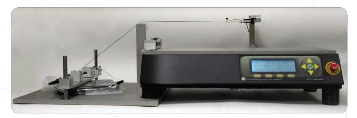
The Thwing-Albert Friction/Peel Tester is the most wide-ranging testing instrument for measuring the coefficient of friction, peel strength, seal strength and tensile strength of flexible plastic films, paper, sheet materials, labels, tapes and textile materials. The tray peel fixture is designed to measure the seal strength properties of rigid trays used in the food and medical industries.
