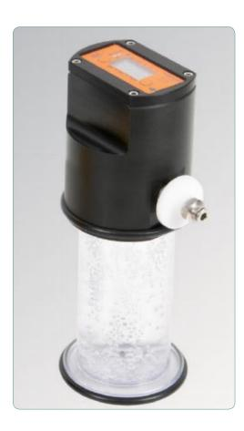
Servicing and adjustment of draught systems for fountain beverages requires robust instruments for quick and accurate carbonation measurement The Steinfurth Cup Carbonation Tester (CCT) combines very easy operation with the new, highly accurate and compact CO2 manometer for simultaneous pressure and temperature measurement as well as CO2 calculation.
