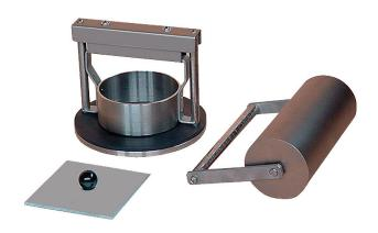
The cobb tester is a simple instrument which measures the water absorptiveness of paper, cardboard and corrugated fibreboard under standard conditions.
