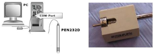
For the programming and read out procedure the pen should be hold near to the center of the T-3T. A special holder making the positioning easier can be optional ordered.
