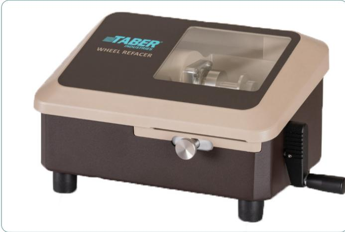
Resurface Taber abrading wheels with precision. The Model 350 Wheel Refacer is used to refresh and standardize the contact surfaces of Genuine Taber Calibrade® wheels when they become clogged with debris. Intended for H-10, H-18, H-22 and H-38 abrading wheels, this instrument can also be used to true out of round wheels and correct 'crowning' conditions on both Calibrase® and Calibrade® wheels.
