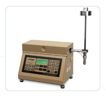
Measure abrasion resistance and other material properties of finished products of any size or shape - flat, concave or convex.
