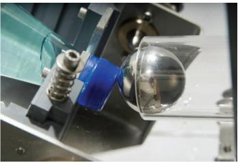
The Ball Impac Tester allows standardized impact tests for bottle closures. The bottle to be tested is held in a box, which can be swung from a horizontal to a vertical position in steps of 5 degrees.
