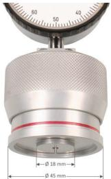
Durometer according to Shore for determining the indentation hardness of soft rubber, elastomers, natural rubber, polyester, soft PVC, leather, etc.
