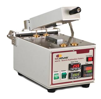
The Scorch Tester determines colorfastness and shrinkage to hot pressing and dry heat. This instrument is available in two different hot plate sizes. The top plate has a unique hinge and spring pin design to ensure even pressure across the sample. Each plate temperature is individually controlled and a timer is integrated with the divice.
