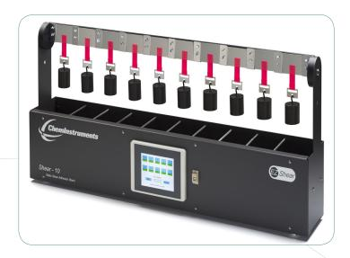
Precise room temperature shear tests are made easier with the ChemInstruments Room Temperature 10 Bank Shear Tester. It performs shear tests according to PSTC-7 Procedure A, TLMI Test No. 7, and ASTM D 3654, Procedure A for holding power of pressure sensitive tapes. It can also be used for PSTC-14, adhesion of pressure sensitive tape to fiberboard at 90° angle and constant stress, and PSTC-7 Procedure B.
