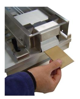
Preparation of corrugated board samples for ECT test
