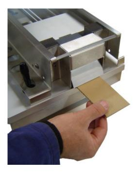
Preparation of corrugated board samples for ECT test.
