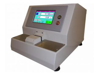
Determination of the compression resistance per length unit in Flutting paper.
