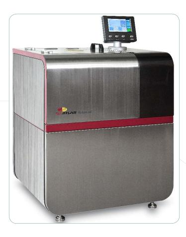
Colorfastness to washing is easy and affordable with the Rotawash. Available in an 8 or 12 washpot model, this instrument can handle either the 550 ml or 1200 ml washpots. Washpots just press into place. The instrument is all stainless steel to provide years of reliable service in a wet environment. The touchscreen controller is preloaded with the most popular tests and provides information on when the test will be completed.
