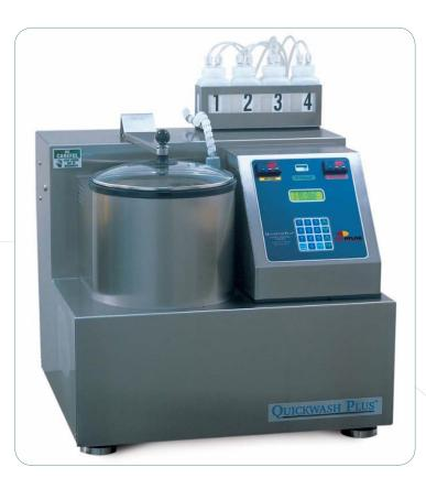
The QuickWash Plus gives fabric shrinkage information in a 12 15 minute test versus the 8 12 hours it takes a standard washer and dryer. This instrument is ideal for the factory floor and provides rapid, on the spot information on fabric in production so that the stenter frame, compactor, and sanforizer can be set to maximize fabric yield. This allows user to bypass the standard wash and dry cycles that take so long thus significantly reducing labor in the lab.
