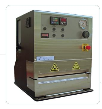
Precision Heat Sealer on an open-back frame featuring a digital timer and temperature controller, surface mounted thermocouple, dual action cylinders, electronic timer activation. The open-back frame allows for both front-to-back and lateral pass-thru capabilities. The standard instrument includes one fl at upper sealing die 1" wide.
