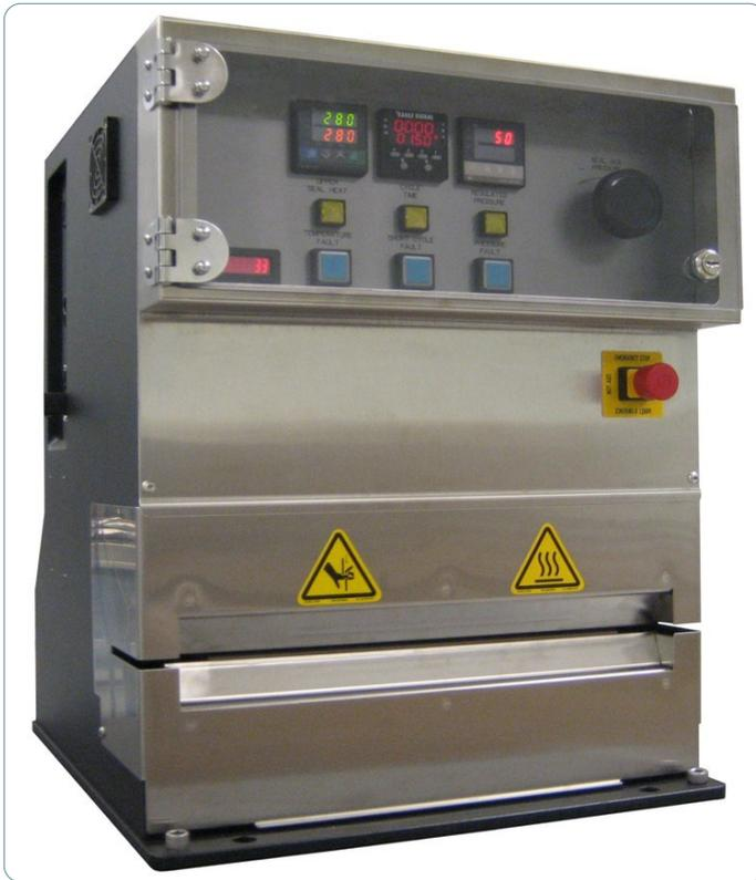
Precision Heat Sealer on an open-back frame featuring a digital timer and temperature controller, surface mounted thermocouple, and dual action cylinders. The open-back frame allows for both front-to-back and lateral pass-thru capabilities. This model offers upper and lower sealing dies (ordered separately)
