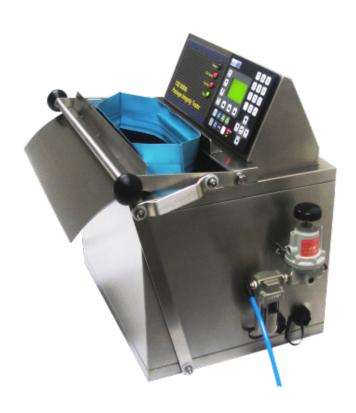
The package integrity tester (P.I.T.) uses a vacuum method to measure the gasleaking from a wide range of flexible pack types and sizes. Items are placed manually into the unit, and the handle is closed to initiate the test sequence. Results are displayed as a Pass or Fail, along with a quantitative measure of the leakage rate.
