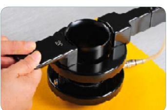
The digital air permeability tester accurately and swiftly determines the resistance of fabrics (woven, knitted and non woven textile materials) to the passage of air (air flow) under constant pre-set air pressure while firmly clamped in the test rig of selected test head/area.
