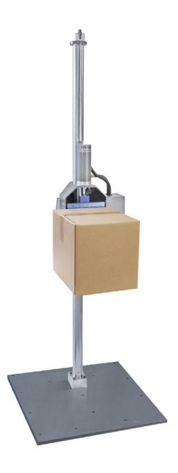
The Model PDT 80M is Lansmont's entry level Precision Drop Tester. The PDT 80M consists of a drop leaf assembly housed in a cast aluminum structure that supports the precision guides and the pneumatic cylinder. This support structure is mounted on a 3 inch (7.6 cm) diameter chrome-plated steel column that is rigidly fixed to the  $\frac{1}{2}$  inch (1.3 cm) thick steel base plate with a heavyduty collar.
