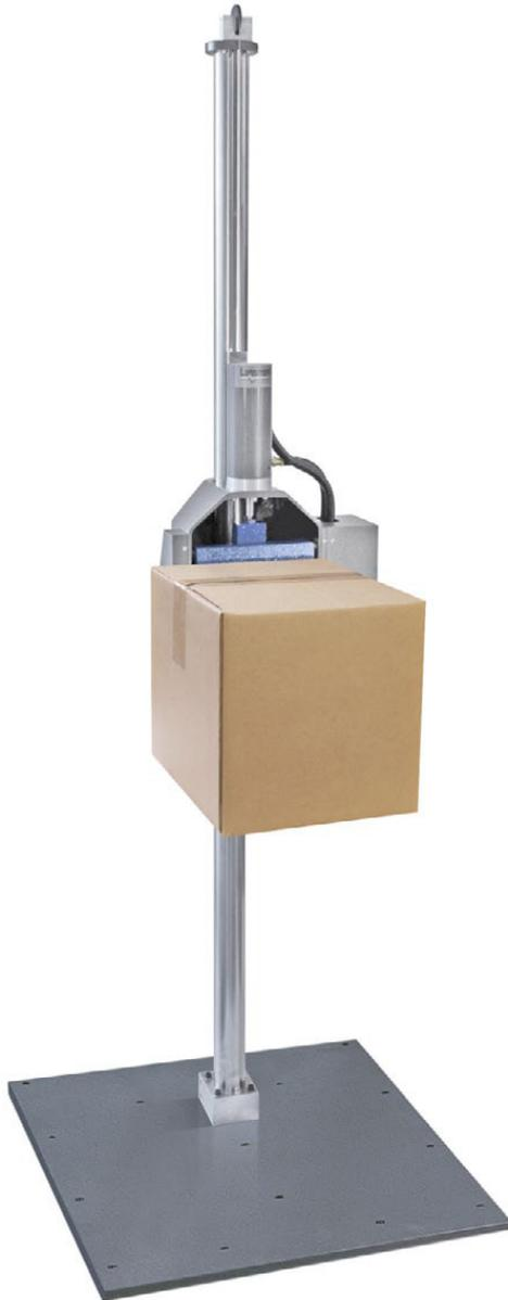
The Model PDT 80M is Lansmont's entry level Precision Drop Tester. The PDT 80M consists of a drop leaf assembly housed in a cast aluminum structure that supports the precision guides and the pneumatic cylinder. This support structure is mounted on a 3 inch (7.6 cm) diameter chrome-plated steel column that is rigidly fixed to the ½ inch (1.3 cm) thick steel base plate with a heavyduty collar.
