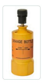
The Orange Bottle is used to verify the operational repeatability of torque measuring instruments. This bottle is constructed with high energy permanent magnets and is pre set at the factory to a customer specified torque of between 5 to 15 inlbs. Each Orange Bottle is labeled with its exact torque rating and repeats to an accuracy of +/- 0.2 in-lbs.
