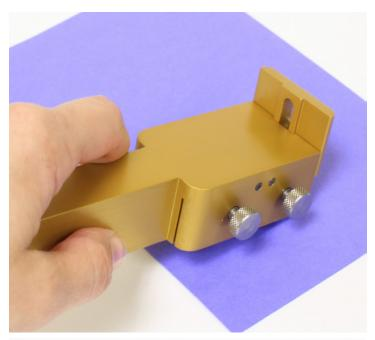
This manual strip cutter can quickly prepare samples of two sizes 1 inch (25.4 mm) or 15 mm for measuring material tensile, peel or seal strength. The cutting blade width is easily adjusted by releasing the blade and moving it to the appropriate slot for the 15 mm or 1 inch strips.
