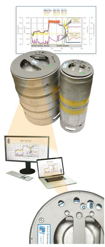
Uses a brewery standard keg fitted with sensors and a data logger. It is an essential tool for every brewery with a keg filling line, large or small. Send it through the line as normal; transfer data to PC or laptop; look at the results on screen and see exactly what is happening inside the keg during every cycle of washing, disinfection, filling.
