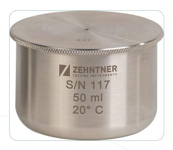
Laboratory apparatus for the determination of the density of coating materials and similar products, in particular liquids with low and medium viscosity at the test temperature.
