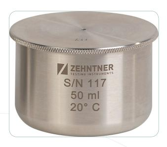
Laboratory apparatus for the determination of the density of coating materials and similar products, in particular liquids with low and medium viscosity at the test temperature.
