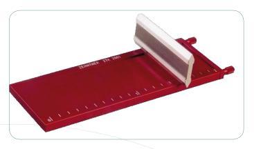
Gauge for testing coating materials and fillers for drying properties, shrinking, mud-crack, cracking and porosity.
