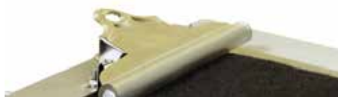
Spring Clip Clamp assembly for holding samples in place.
