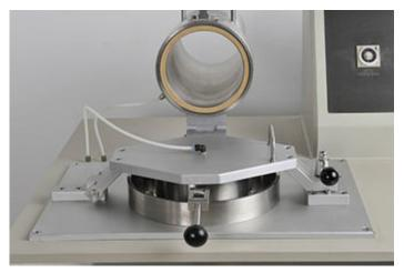
Automatic sheet former has the same system as the manual one. With 159 mm sheets. This equipment avoids the error by human factor in the sheets production practically in its entirety. With operations of filling, agitation, calm, emptying and automatic drainage. Removing the sheet without roller by vacuum system. To finish the formation of the sheets, a press and a quick dryer are necessary.
