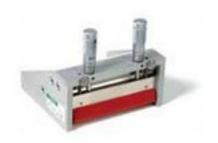
This film applicator includes two integrated micrometric screws to adjust the height of a knife. The distance of this knife can be adjusted in steps of 10 microns from 0 to 6 mm. Produced in hardened stainless steel.
