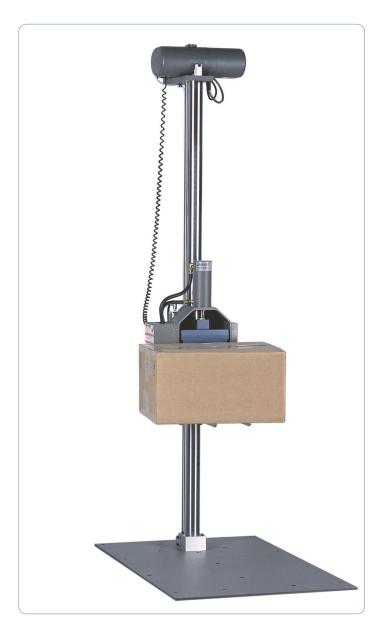
The transport and distribution environment holds numerous opportunities for packages to experience impacts and/or drops. As a result, shock is transmitted both into, and throughout, a given package. The products within the packaging respond to both the amplitude and frequency characteristics of the shock. How the various packaging components mitigate that shock determines how much shock is transmitted into the product held within.
