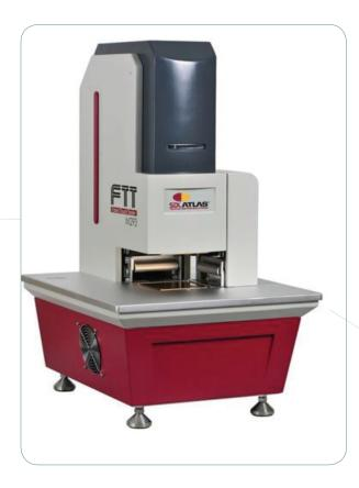
The innovative FTT measures skin touch properties of textiles objectively and quantitatively. The comprehensive, sophisticated design of the FTT enables it to measure all the mechanical and surface properties of fabric in one simple test. Previously only possible on the very expensive and technically complicated Kawabata instruments, the FTT now makes hand measurement possible for everyone.
