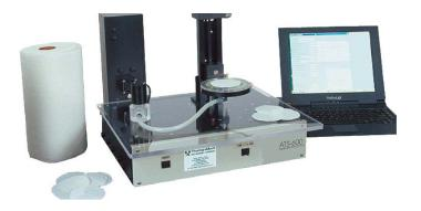
This absorbency testing system is ideal for research and development as well as quality control applications. Its small size and rugged design make it suitable for both the laboratory and the production floor. It is a table top instrument that measures the absorption desorption rate and total capacity of absorbent materials in real-time.
