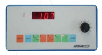
User friendly key panel for selection of test method (A, B or C), twist direction (S or Z) setting of moving clamp rotation speed by means of a potentiometer and data transmission to the printer.
