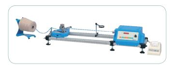
Electronic Twist Tester to determine twist of single, twisted (S&Z) and Open End yarns. Three methods available to be selected by the operator:
