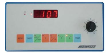
User friendly key panel for selection of test method (A, B or C), twist direction (S or Z) setting of moving clamp rotation speed by means of a potentiometer and data transmission to the printer.
