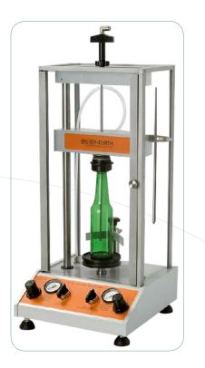
The Steinfurth Sampler pierces and pressurizes bottles and cans. Piercing and sampling is performed pneumatically, so there is no need for great manual forces. Fully automatic operation makes beverage sampling even very simple. The Steinfurth Sampler is suitable for gas analyses (e.g. oxygene, CO2,...) and foam stability measurements.
