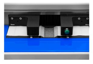
Water bath for wet tensile measurements. Measurements for up to 50 mm wide stripes possible. The tensile test ranges from 50 mm to 180 mm distance between the clamps.
