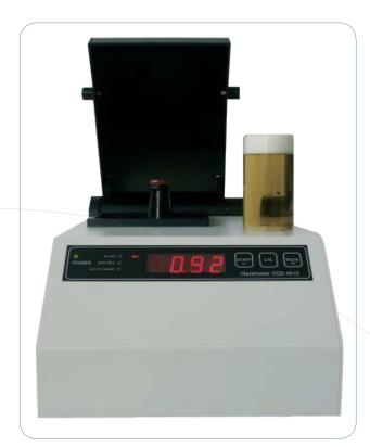
Turbidity is defined as "expression of the optical property that causes light to be scattered and absorbed rather than transmitted in straight lines through the sample." In other words, turbidity is the measurement of relative sample clarity. Turbidity is measured by comparison to standard solutions eg. Formazin.
