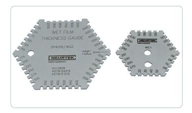
Wet Film Thickness Gauge WG is a hexagonal/octagonal precision measuring comb made of heavy stainless steel. The high-grade stainless steel will not be affected by acid or base elements. Models available for several different applications.
