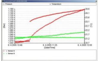
The Steinfurth pressure transmitter system type DH is a means to measure and record absolute pressures inside closed PET bottles over a long period of time.
