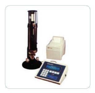
Densometers are the accepted standard for measuring the porosity, air-permeability or air-resistance of sheet-like materials such as papers, wovens, plastics and mebranes. Certain models such as the S-P-S Tester are also used to measure surface smoothness and material softness. Manual and automatic units are available.
