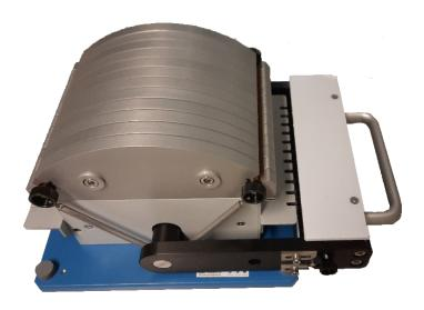
The film-/paper Strip Cutter was developed to cut over for instance DIN A 4 large film or paper sheets up to 10 pieces parallel strips in one processing step. These strips can be used for further evalutations (e. g. tensile strength, tension, elastic module, etc..) in accordance with the international standards.
