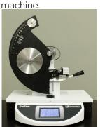
The touch-screen display allows for quick clamping and testing. Lab technicians can easily customize units of measurement to their screen preference. Other functions include data entry of sample information such as sample ID, thickness, basis weight, sample direction and number of plies being torn.
