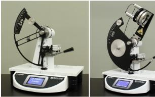
Thwing-Albert is the original manufacturer of the Elmendorf Tear Tester which was designed by Dr. Thwing and Mr. Armin Elmendorf. This method developed over a century ago established the industry standards used worldwide today to measure tear strength.
