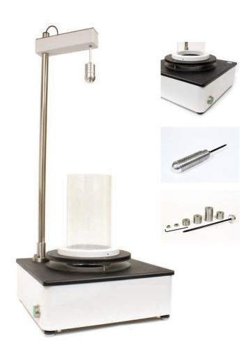
The dart drop tester is an easy-to-use, ergonomically designed instrument used to measure the impact resistance of plastic film, coated paper and other materials.
