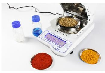
The CrystalTherm Infrared Moisture Analyzer has been designed to be used in the food, industrial, professional or laboratory sectors. It determines the dry matter after the drying process of the previously weighed sample. During the process you can see the decrease of the moisture content on the display. It is also an ideal analytical tool to accurately determine the consistency of materials and volatile and fixed substances.
